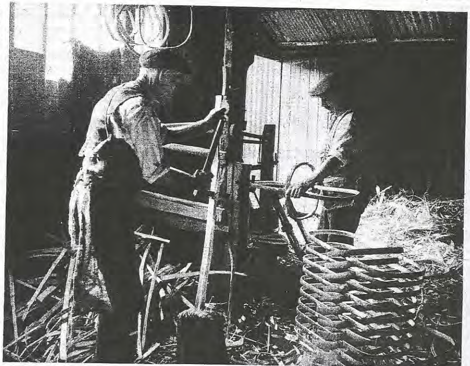
The making of trugs, those long, shallow baskets used by gardeners and greengrocers, has been practised for centuries in Sussex. The picture shows two craftsmen at Hurstmonceux bending the frames. Times
