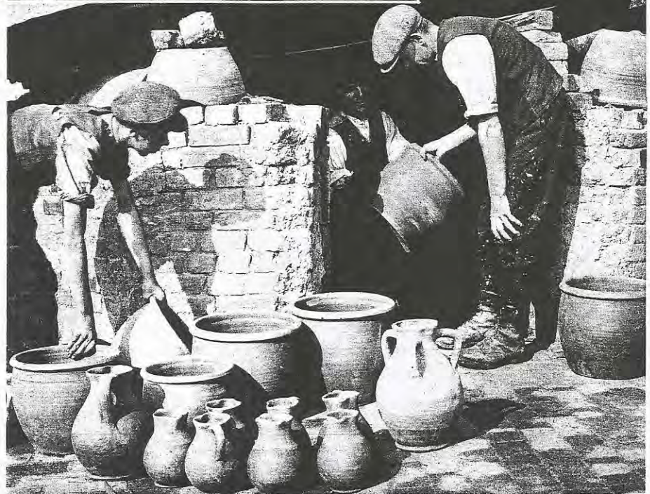
This hand pottery at Verwood, Dorset, is about 200 years old. In the upper picture a boy is seen working the revolving throwing-table while the potter throws his pitcher or bread-pan—the chief products of this pottery. The lower picture shows the dried pots and pans being placed in the kiln for baking.
