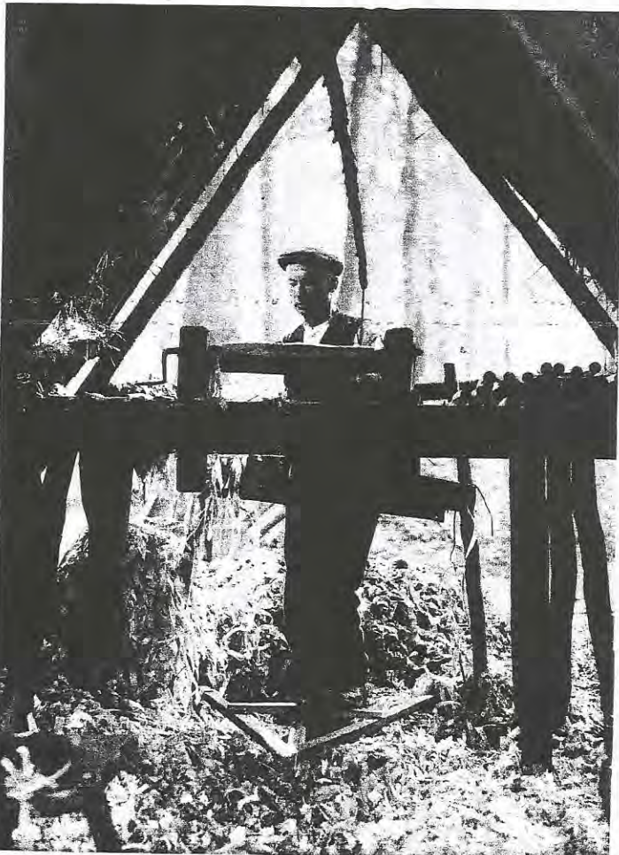
Chair bodgers, as they are called, are associated with the Chilterns. Many of them work in rough sheds in the heart of the woods. This craftsman is turning a chair-leg on a pole-lathe. Times
